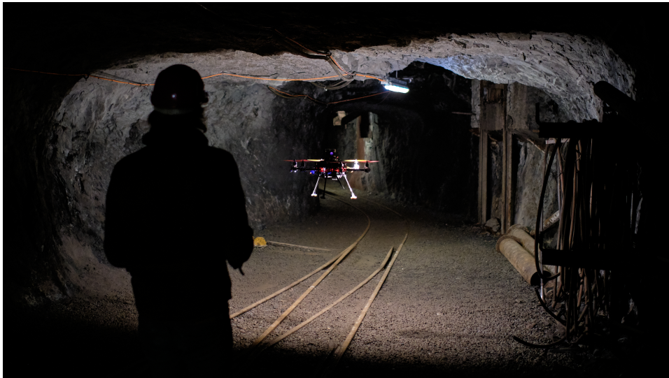
Figure 1.1: The quadrotor is deployed to make a map of the tunnel. With a limited battery capacity, it needs to travel the unknown area fast and efficiently while building a map.
